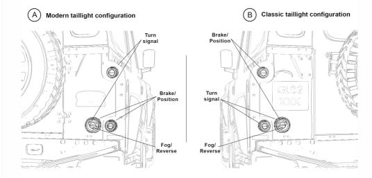
The GL-2 .1 taillight is a sided taillight indicated by an "L" for left "R" for right and top facing installation indicated by 2 arrows on the housing. It is important to install the lamps on the correct side and facing up.
